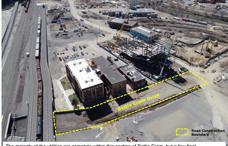
The majority of the utilities are complete within this section of Bettie Cram, but a few final connections are underway seen here with the large trench. Preparations are underway for paving.
